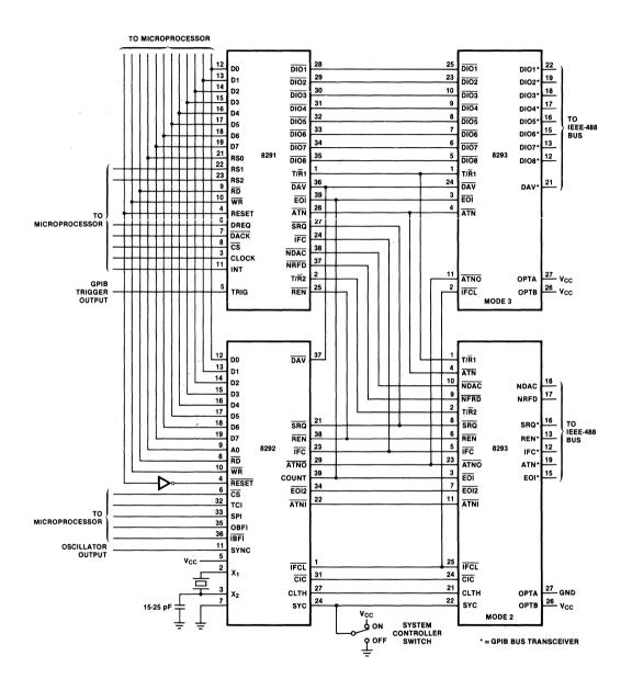
Figure 8. 8291, 8292, and 8293 System Configuration
